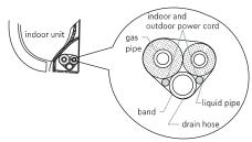
2. Reserve a certain length of drain hose and power cord for installation when binding them. When binding to a certain degree, separate the indoor power and then separate the drain hose.
