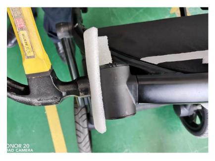
4. To add glue on screws and fix new front caster assembly by new screws
