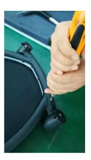
2. Using foam protect tube, knock caster by rubber hammer to remove casters; and scrap them.
