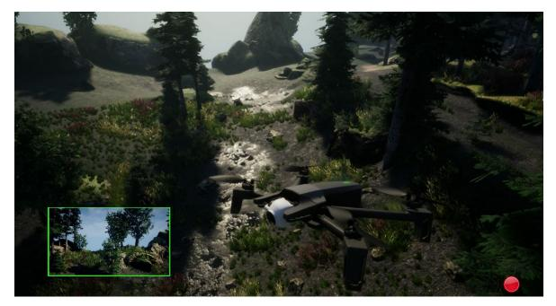
ANAFI USA's firmware, as simulated on an emulated hardware (camera, sensors and actuators), is identical to ANAFI's actual software. The simulator allows automated testing (headless) and alteration of a hardware peripheral, in real time.
