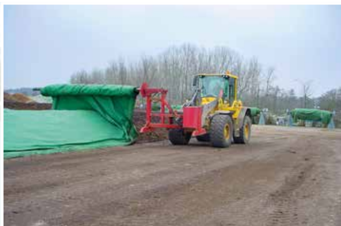
High tensile strength allows to roll and unroll the fleece with mechanical arm or compost tuner.
