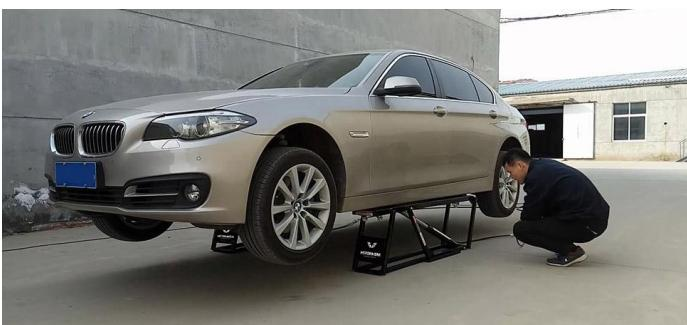
Press the "Down" button to fully lock the mechanical lock and start maintenance work
