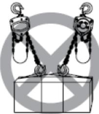
3. NEVER use two or more hoists together to lift load beyond the rated capacity of hoist.
