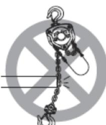
5. NEVER run the load chain over a sharp edge.
