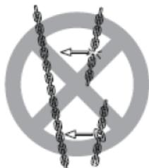
1. NEVER use a twisted, kinked, damaged or stretched load chain.
