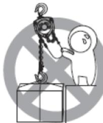
4. NEVER lift up load beyond the rated capacity of the hoist.
