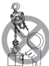
6. NEVER weld or cut a load suspended by a hoist.
