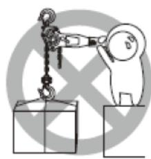
4. NEVER lift up load beyond the rated capacity of the hoist.
