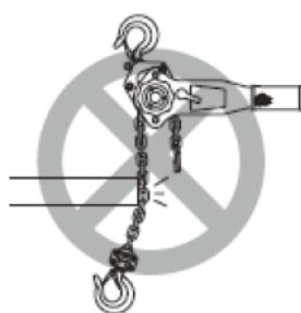
5. NEVER run the load chain over a sharp edge.
