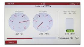
The volume flow is shown as I/min on the display, as well as the test pressure. In addition, the leakage is given in percent. The maximum permissible leak rate is 100%.
