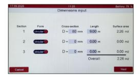
After selecting the pipe measurements, press "continue" to start the actual measurement. The device will then self-test and calibrate. Then the measurement menu appears. After the test pressure has been built up, the measurement will start over a period of 1 minute and finally shows the result as an average value.
