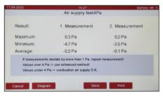
Two measurements (each 4 minutes) will be carried out and the result displayed. A tip is issued for the measurement result. Under "Graphics" a graphical history can be displayed.
