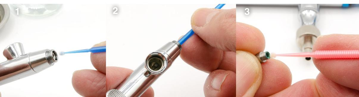
1, 2 & 3. Prolonged use of the airbrush causes paint to be deposited inside it and may clog it completely. It is advisable to disassemble and clean this tool at least once a month. They will allow access to clean difficult areas in a simple and comfortable way.
